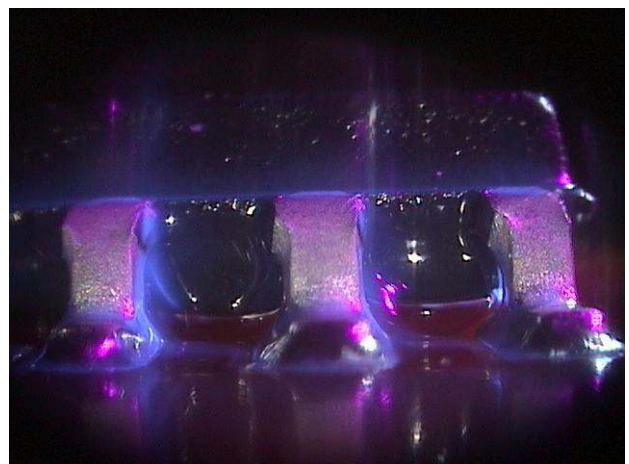
Satisfactory Coating under UV Light
