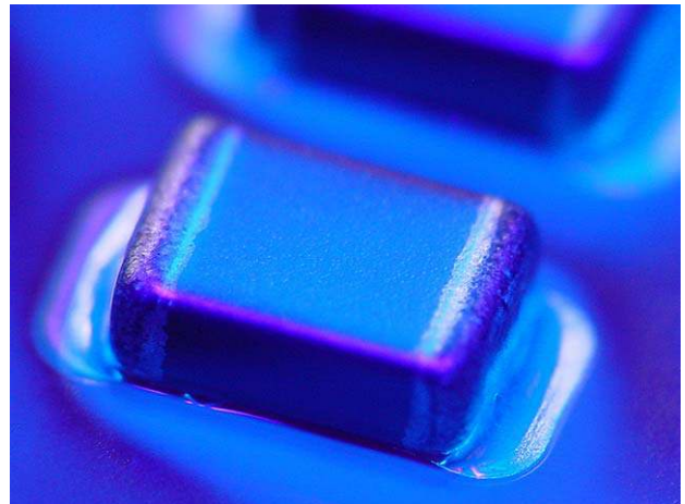
Satisfactory Coating under UV Light
